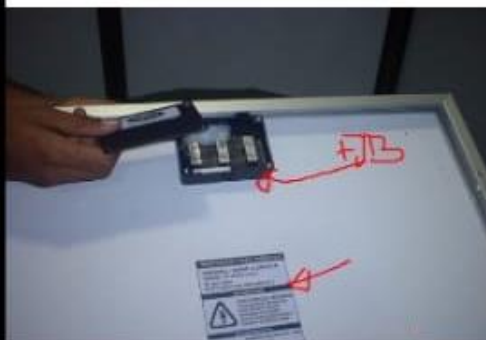
Fig. (i): Opening of module junction box Fig. (ii): Module cable with correct polarity
