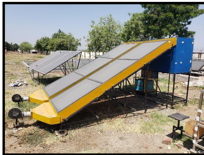
Solar Dehydration System with energy storing material for Agricultural Products
